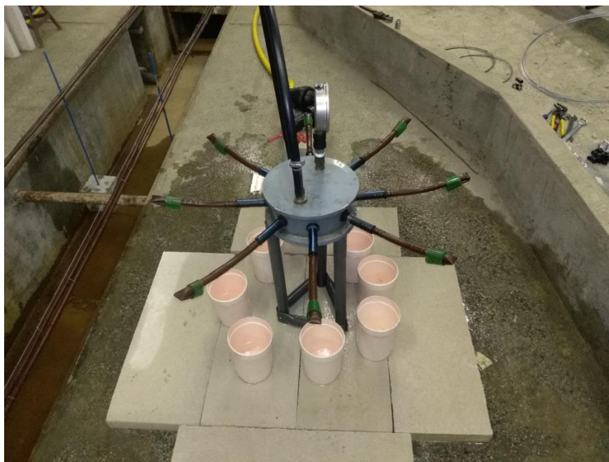
Fig. 5. Experimental setup for determination of flow rate vs. pressure relationship of drippers
