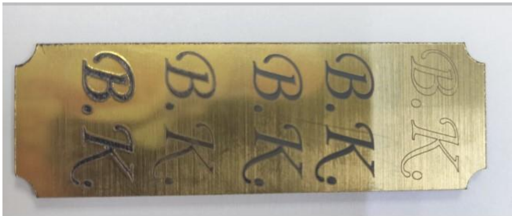
Fig. 4. Two-layer ABS (Acrylonitrile Butadiene Styrene) sheet suitable for laser engraving
