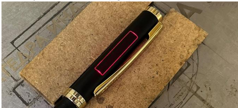
Fig. 2. Marking the print field according to the desired size and position
