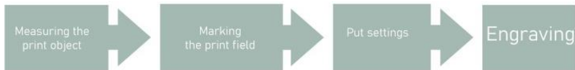
Fig. 1. Methodology of laser engraving process
