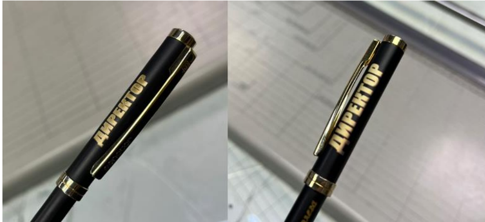
Fig. 3. Engraving on identical objects with a change in the marking field size
