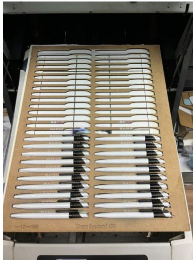
Fig. 7. Physical matrix for multiple use, made of plywood to optimize the process in printing pens
