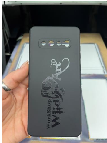
Fig. 4. Printing a logo on a silicone phone case by adding selective lacquer
