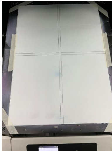
Fig. 6. Graphic template incorporating the dimensional shape of the object, distributed over the printing area of the machine
