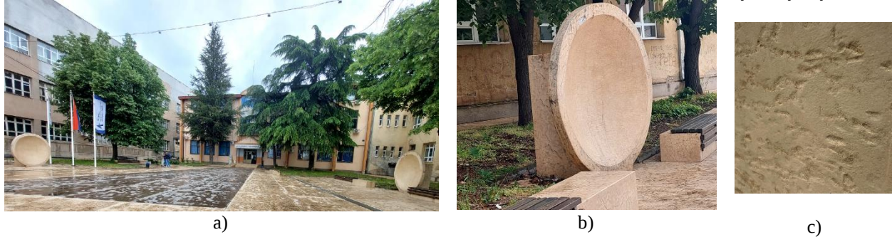
Fig. 1. Acoustic parabolic reflectors: (a) system of coupled acoustic reflectors (Refl. 1 and Refl. 2); (b) view of parabolic reflector 1 (Refl. 1); and (c) detail of the surface roughness of the reflecting surface of Refl. 1.
